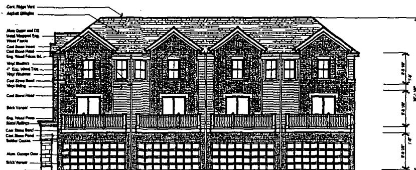
Typ. Side Elevation Exposed Facade 3/16" = 1'-0"
